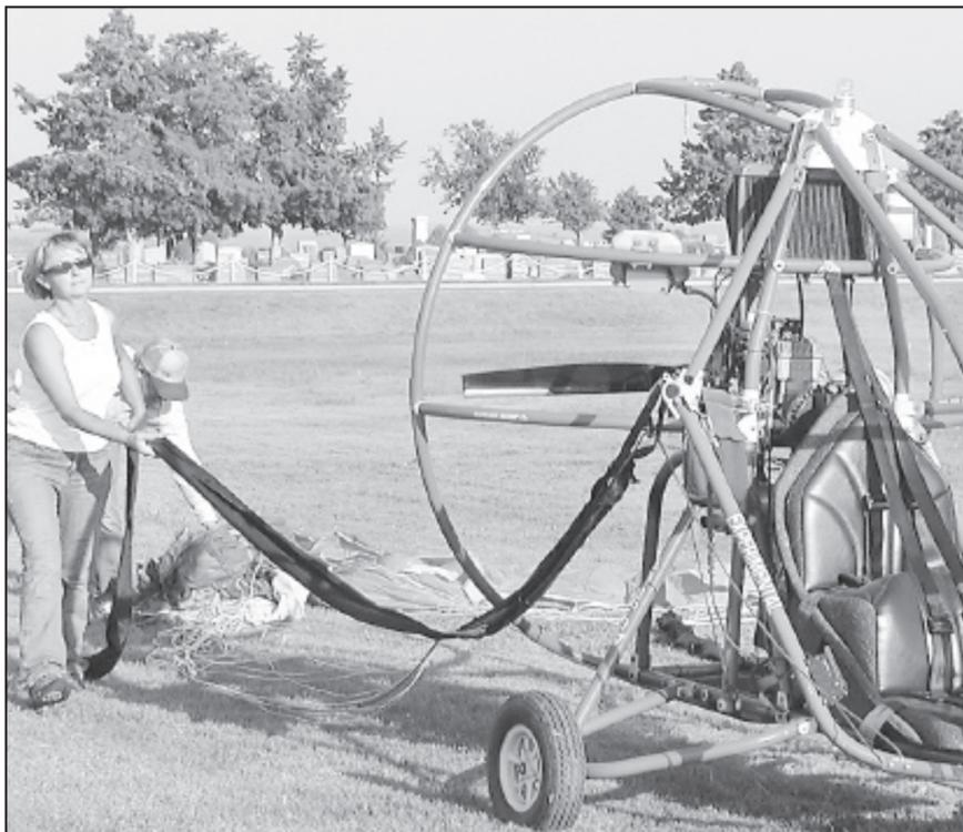
Donna and Steve Tanner lay out the parachute and lines to get ready for take-off. It is driven at about 30 miles per hour until the parachute rises enough to lift the entire unit off the ground. — Photo by Brandy Leroux
