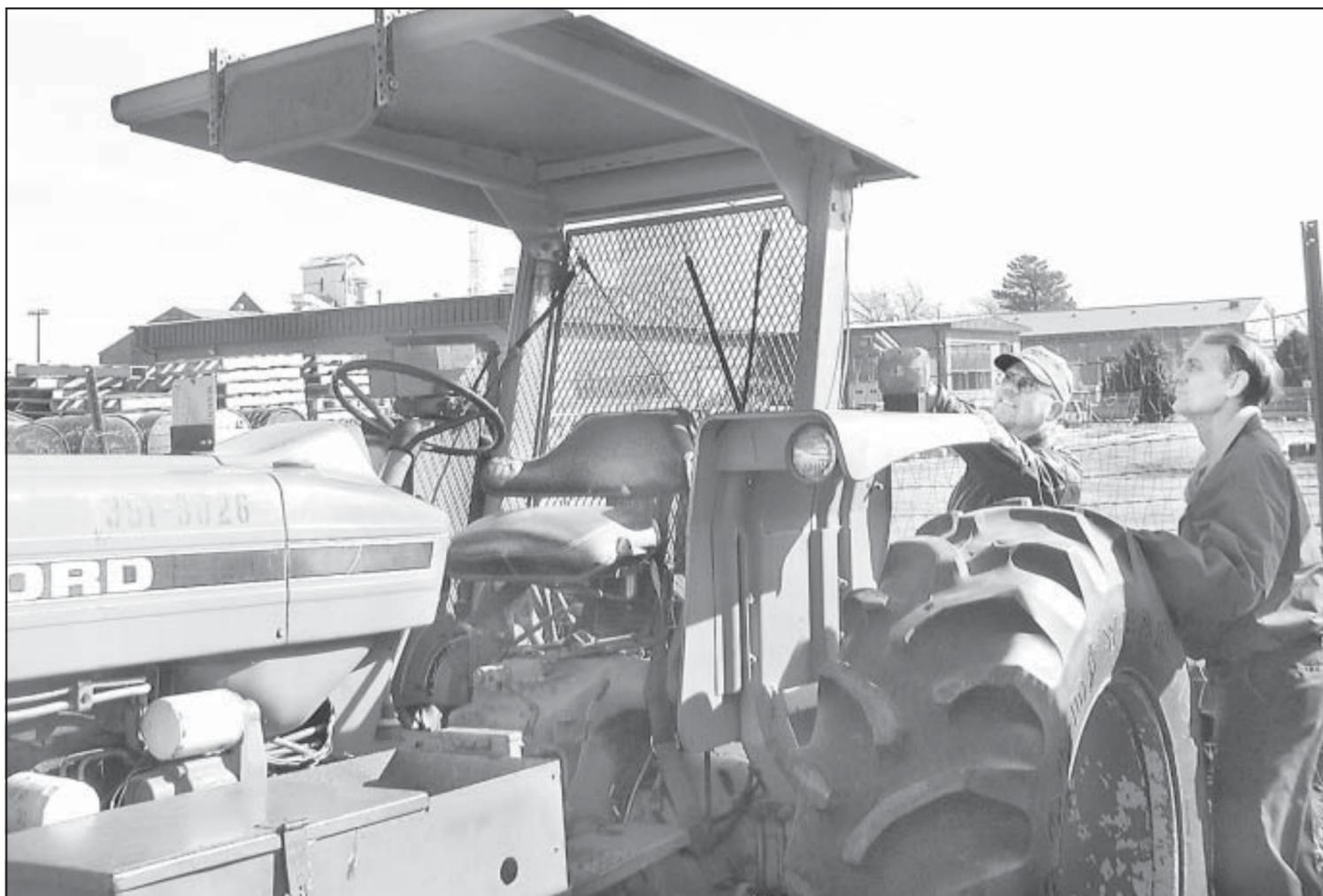
Farm Bureau member, Jon Lofgreen, (above left) and Roy Skrdlant, of Roy's Sales and Service, Norton, inspected a tractor's safety features including a seat belt and rollover protection.. The men (below) look under the fender of a tractor to see if a rollover protection structure, like the cage on the tractor in the top picture, could be added.
