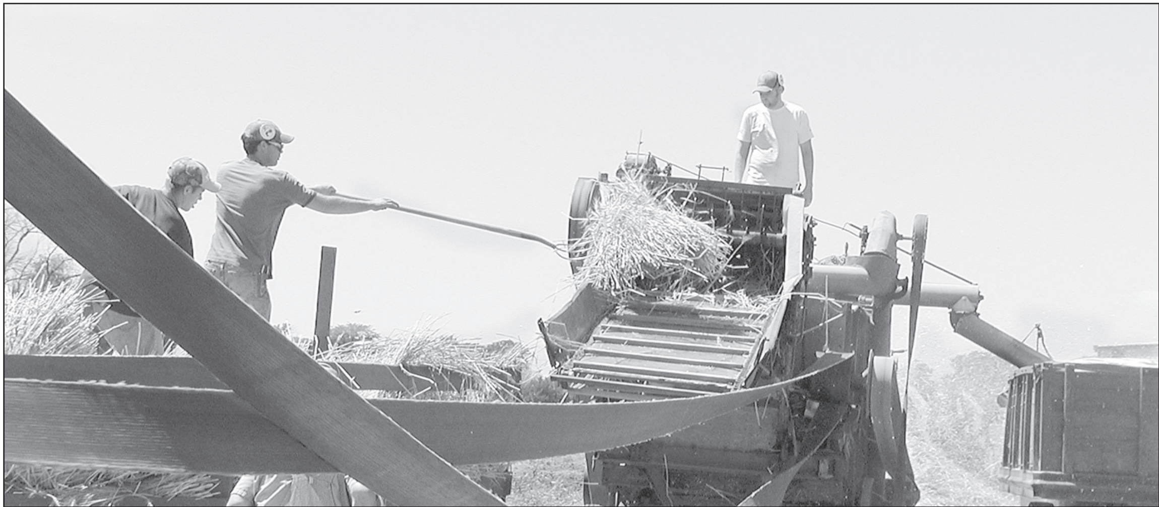
Volunteers at the Tri-State Antique Engine and Thresher show in Bird City piled wheat from a wagon into an old belt-driven thresher during a demonstration of how things used to be done in High Plains fields. The wheat had been cut by a reaper and then the grain had to be threshed or separated from the stalks and chaff. Today, a single machine combines the three jobs. Photo by Bird City Times
