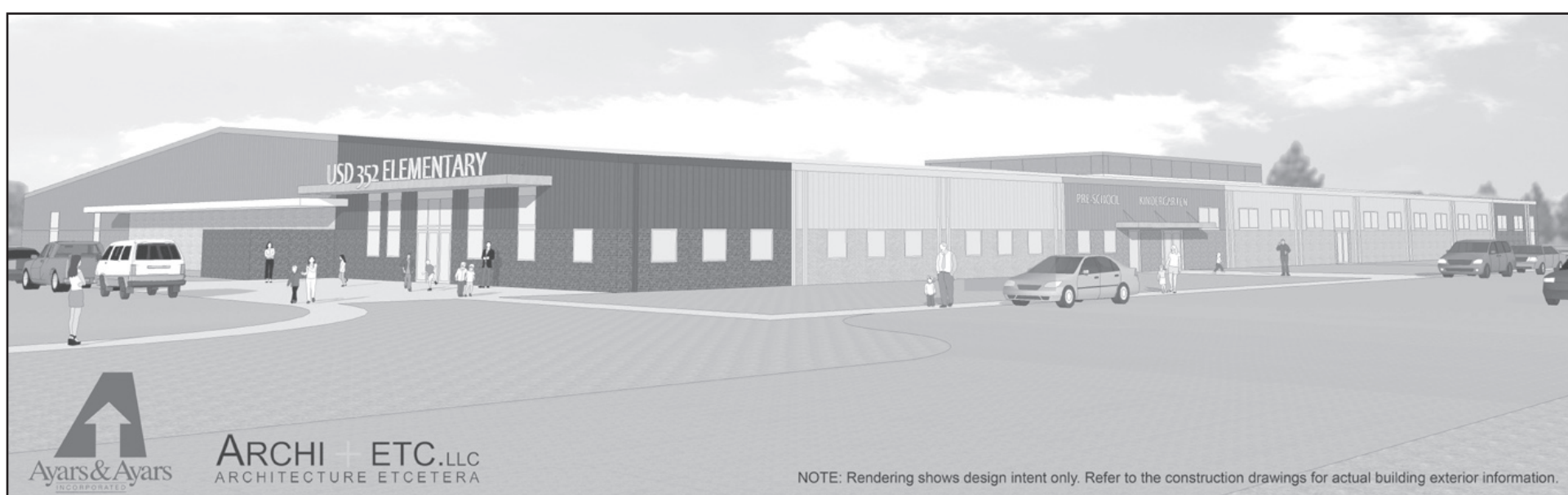
Proposed architect rendering of the new North K-6 building with the mainentrance to the west and a special entrance to the south for the Pre-school and Kindergarten. Buses would drop students off on the east side. The school board decided to go with a full brick outside to reduce maintenance cost and damage from hail.
