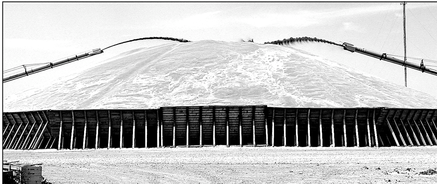
Augers unloaded wheat from trucks on either side of a wheat pile at Frontier Ag in Goodland last week and added it to the pile.
