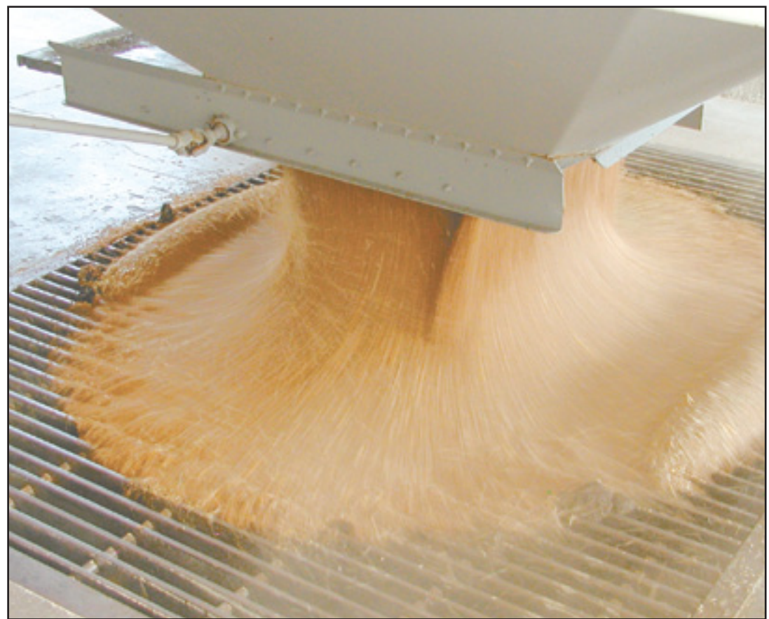
GOLDEN WHEAT is being dropped from the hopper trailer into the pit to be transferred to the storage bin at the Wheeler Equity.
