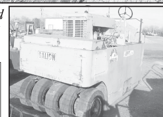
Gallion Rubber Tired Roller 9P-12G-4964 6 Cylinder, 3 Speed
