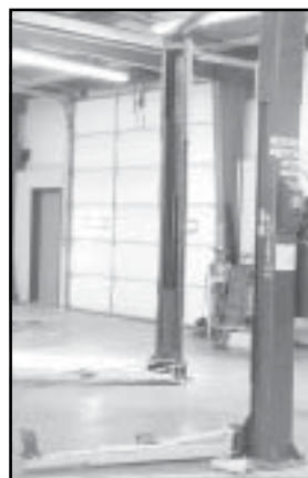
2 Rotary Model SPOA 9 200 Lift, 9000 Lbs. 220V, 2 HP
