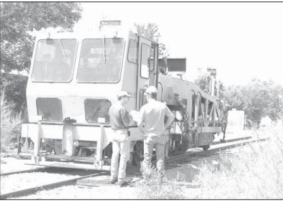
Monsters roared down the rails in Norton on Thursday as track crews for the Kyle Railroad used a "tamper" (right) to lift rails and ties and a "ballast regulator" (above) to straighten the alignment of the tracks, fill in holes and reshape the ballast. The machines can fix one and one-half mile of track a day. - Staff photos by Cynthia Haynes
