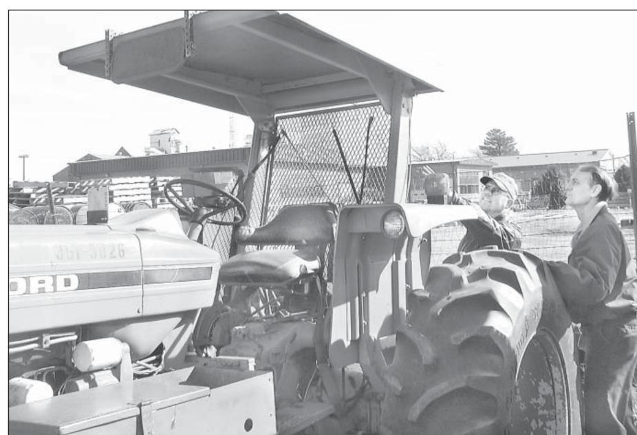
Farm Bureau member, Jon Lofgreen, (above left) and Roy Skrdlant, of Roy's Sales and Service, Norton, inspected a tractor's safety fea-structure, like the cage on the tractor in the top picture, could be tures including a seat belt and rollover protection.. The men (be- added.
