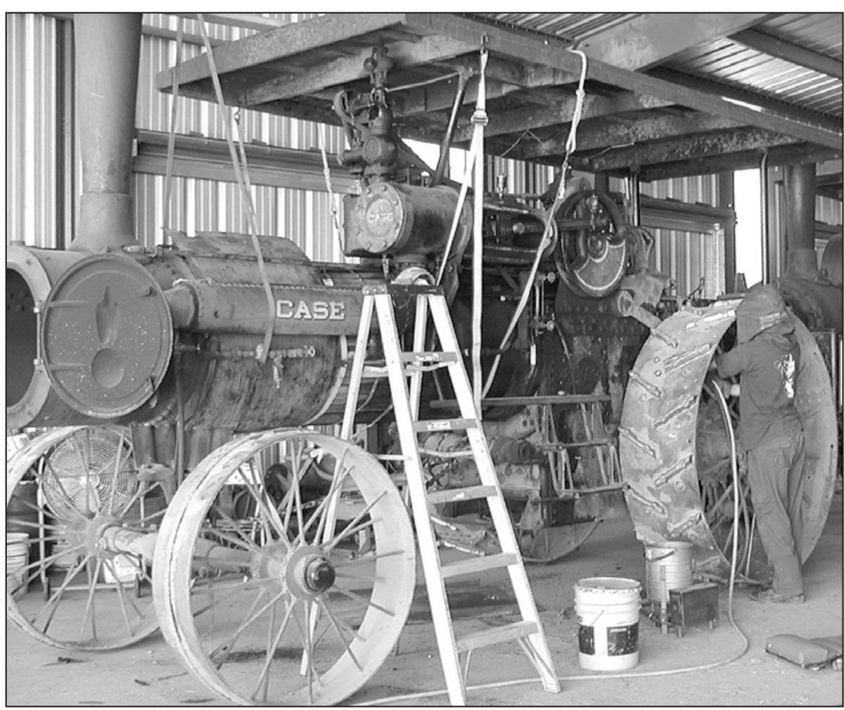
LLOYD STOVER from Pueblo, Colo is sandblasting spots for the ultra sound to test the boiler thickness.
