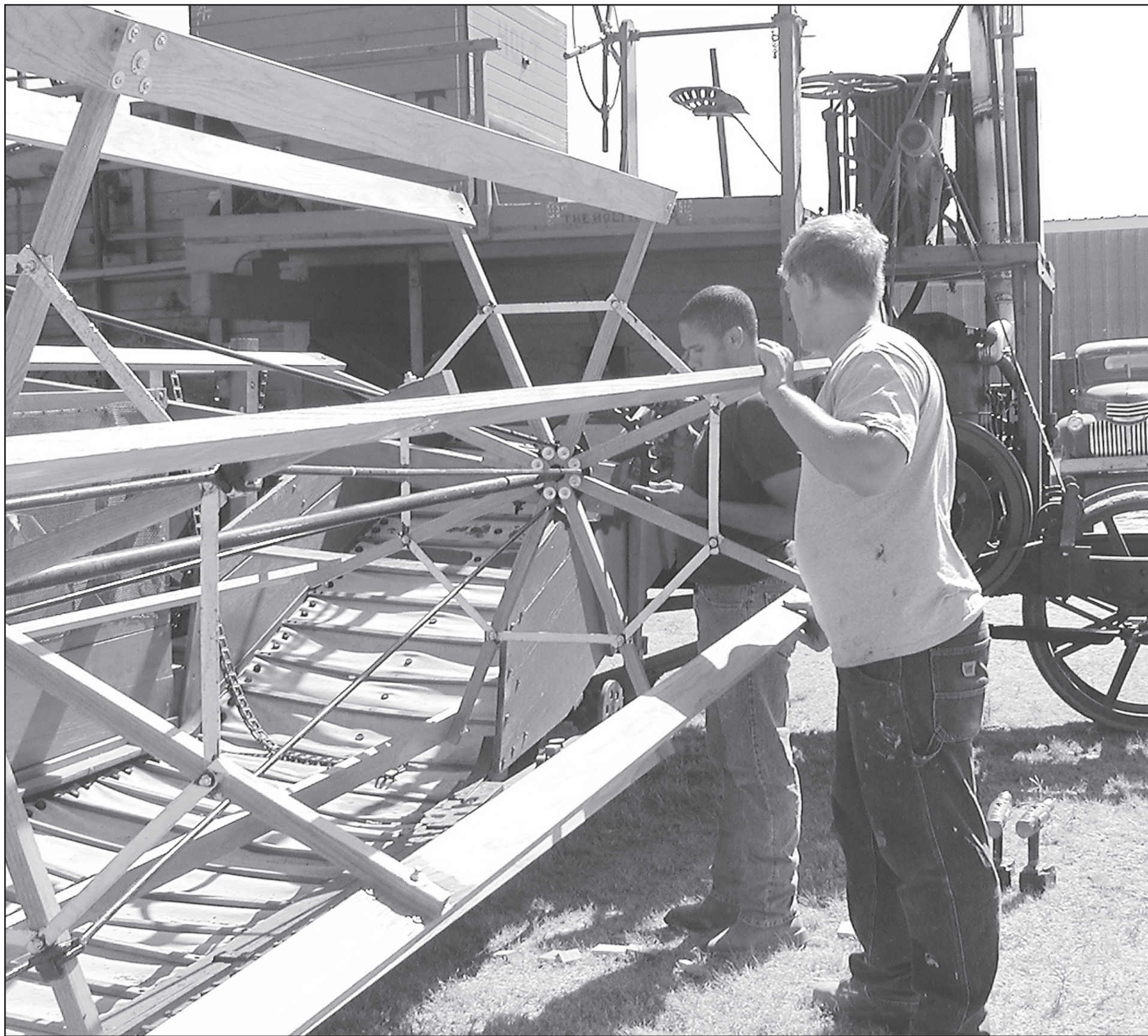
ALAN Burgess and Walter Zarbowski are adjusting the gears on the re-built stroke system to the 1922 Holt Combine.
