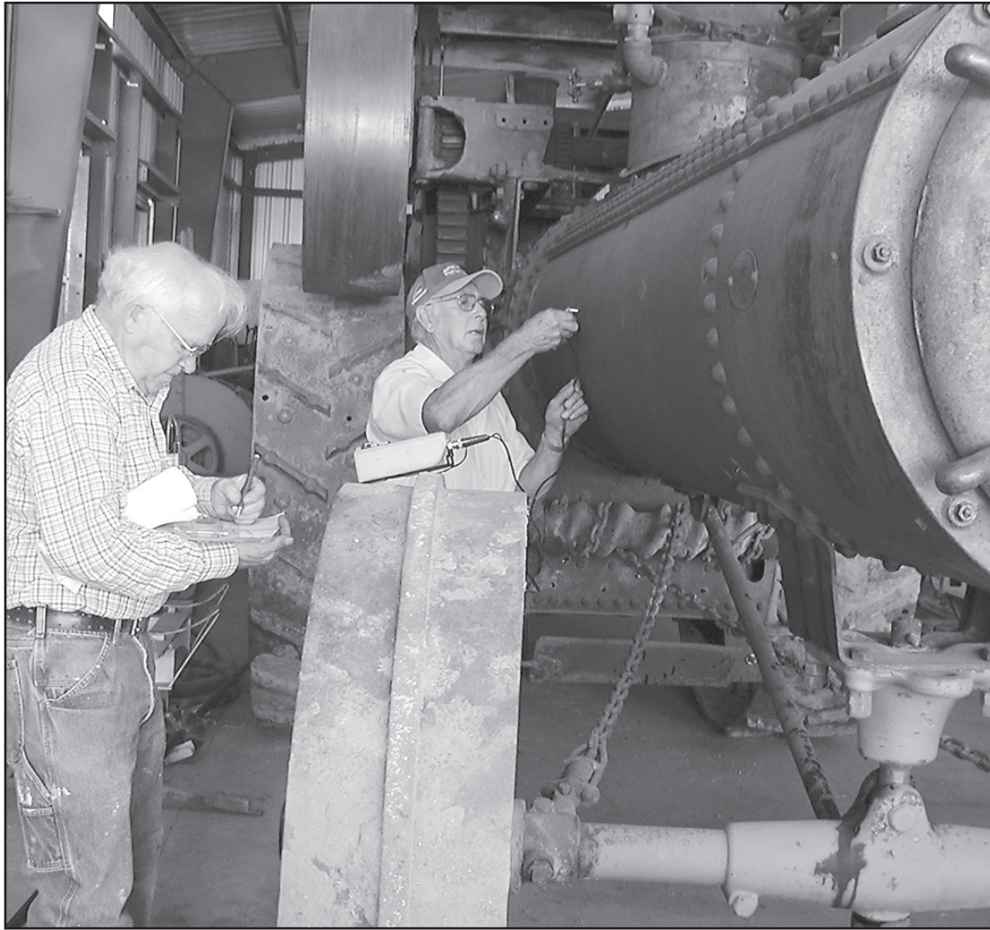
GERALD WRIGHT is teaching Ray Martinez his apprentice worker how to do an Ultrasound. They are measuring the thickness of the boiler plate on a 1914 Case 65 horse threshing machine belonging to Dennis Paden in Norton. Times staff photo by Norma Martinez
