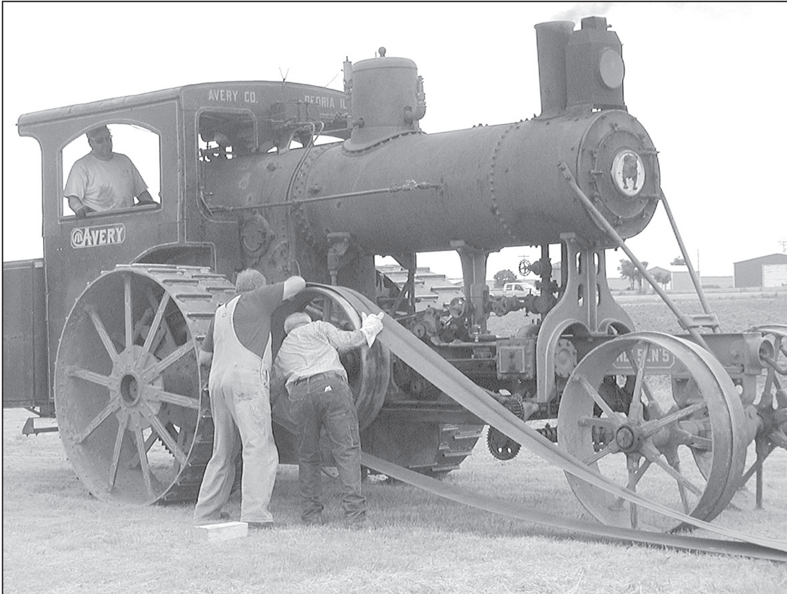
GETTING READY — Mike Levin, driving, Lynn Osburn and Arnold Wright put on the belt from the thresher on the steam engine.
