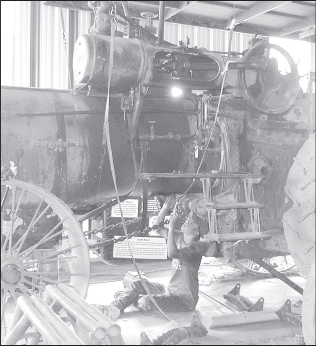
MARCUS COLSON IS GAUGING the boiler of this steam engine to check for safety before it can be certified for insurance. All the steam engines must be certified before they are allowed in the parade at the Tri-State Thresher Show.
